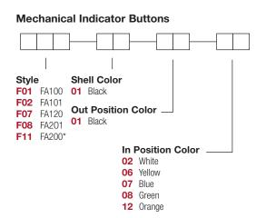
\*Button options for central mounting configurations, use 'FG' for central mount with chrome dress nut, use 'FA200' for central mount with black dress nut.
