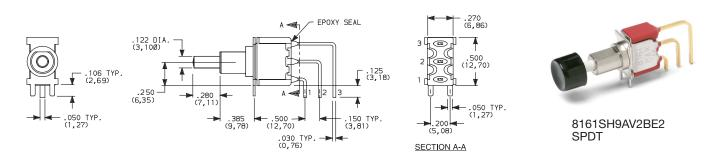
AV3 VERTICAL RIGHT ANGLE, SNAP-IN, PC THRU-HOLE, .150" PITCH
